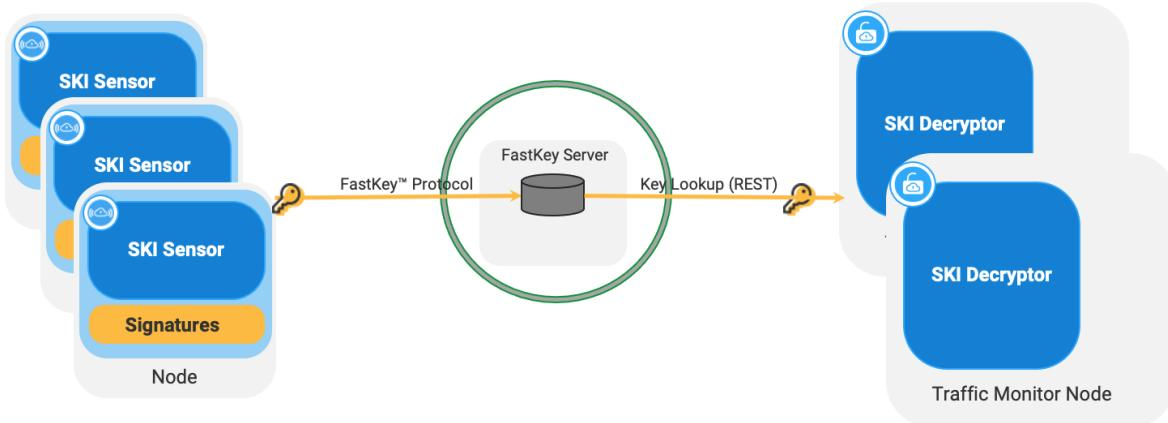
The following figure shows a FastKey Server receiving keys from multiple sensors and returning keys to a *SKI Decryption Library*.
