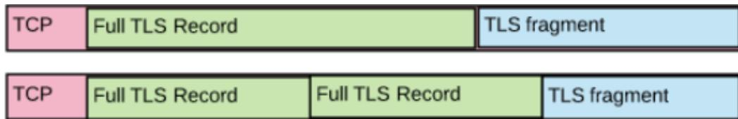
`nu_record_processor()` outputs the decrypted data from all the TLS records in the outdata buffer, and `len` is set to the length of the decrypted data. The return value is `RECORD_NO_ERROR`, indicating that more packet payload inputs are required to complete the next TLS record.
